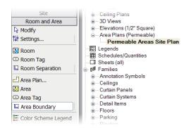
To create a new Level 1 area plan of the permeable area scheme type you just created, click View menu > New > Area Plan. Do NOT associate lines with exterior walls when prompted. Use the option bar filter to copy just the detail lines from the Level 1 floor plan. To place them in the Permeable Areas Site Plan, click Edit menu > Paste Aligned. Click View menu > Properties. Finally, select Level Below from the lists under Primary Range Bottom and View Depth Level.
